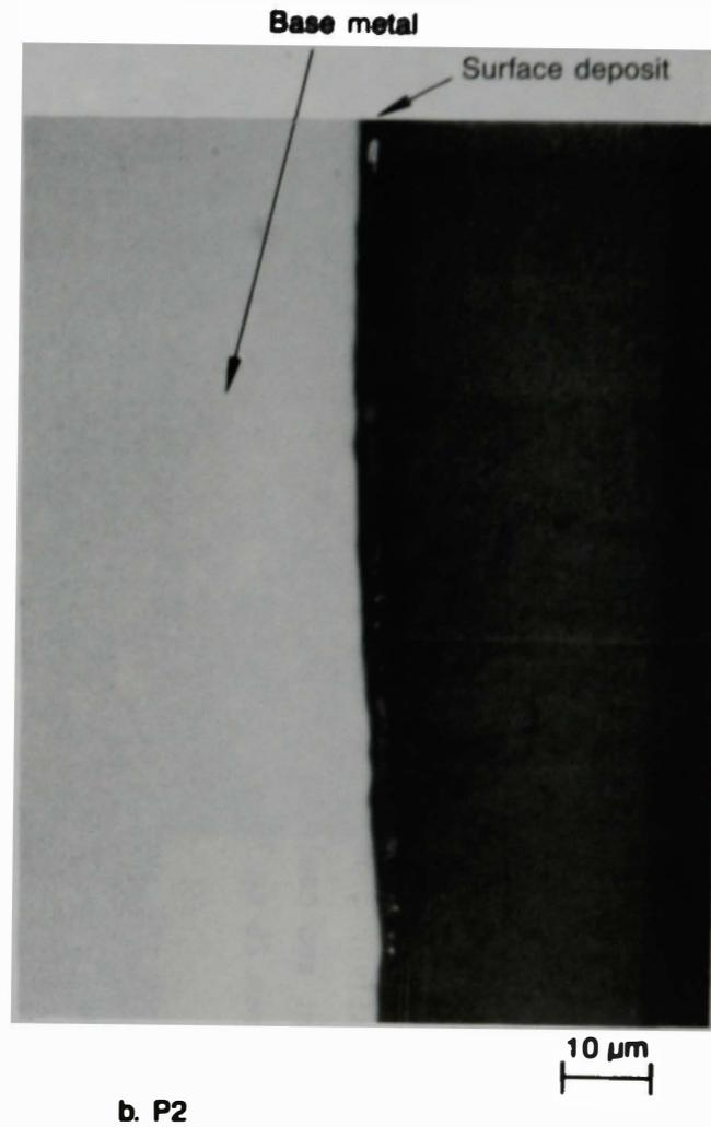
Figure 16. Optical micrographs of specimens from Plate P.
