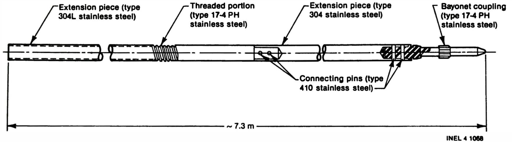
Figure 6. A schematic of a control rod drive leadscrew.
