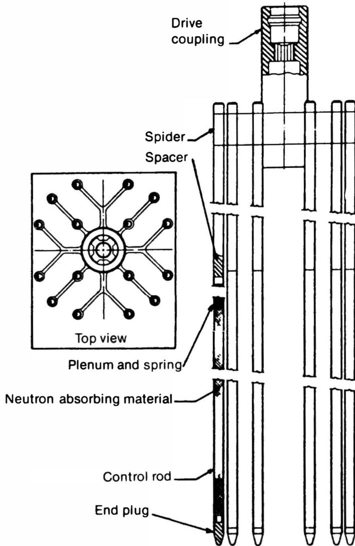
Figure B-4. Control rod assembly (from Ref. 8-1).
