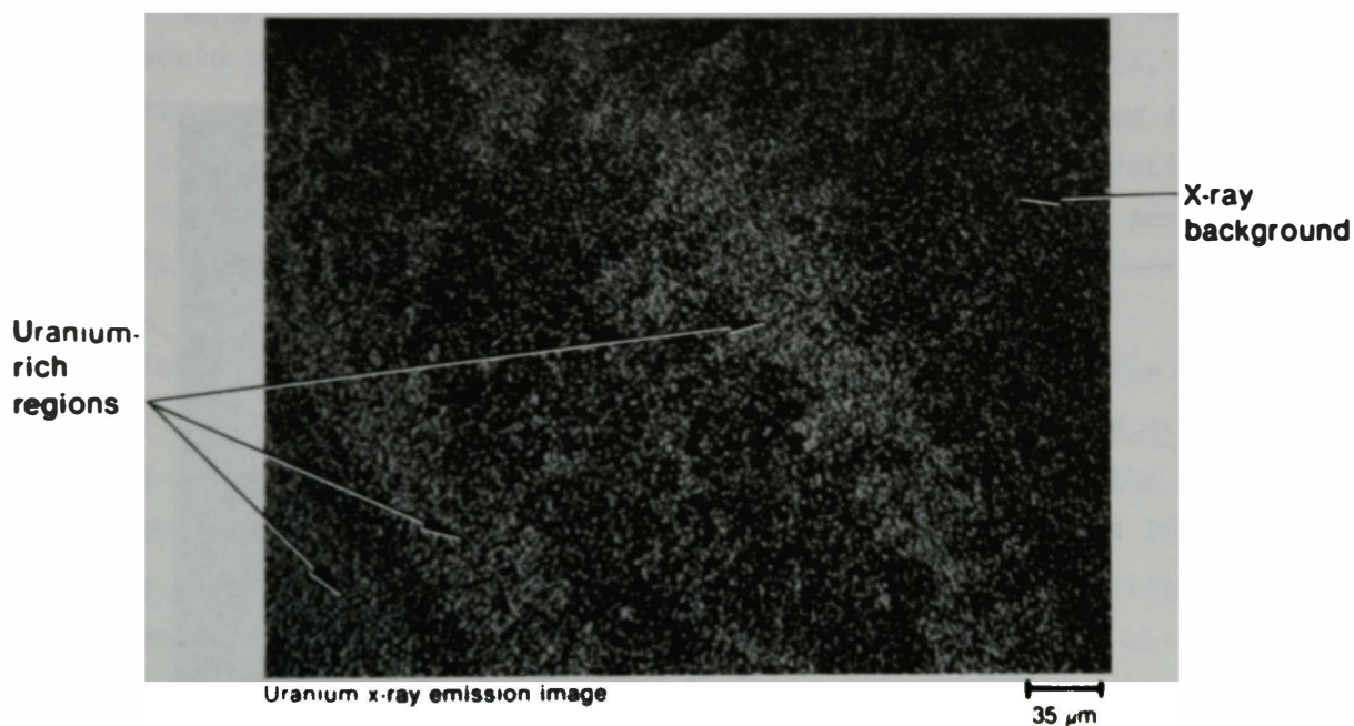
Figure 18. Multiple forms of U, Zr, and O segregation upon cooldown of a heterogeneous melt near the fuel-cladding interface in Particle 1E.
