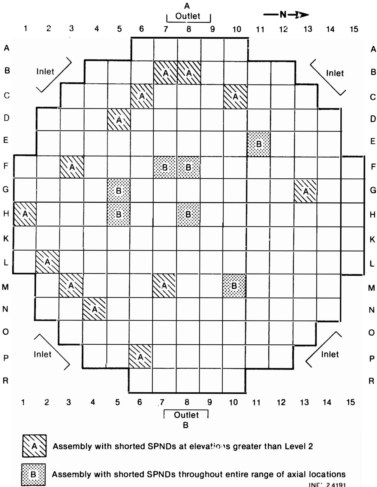
Figure 10. Thermal damage estimates for TMI-2 in-core SPNDs.
