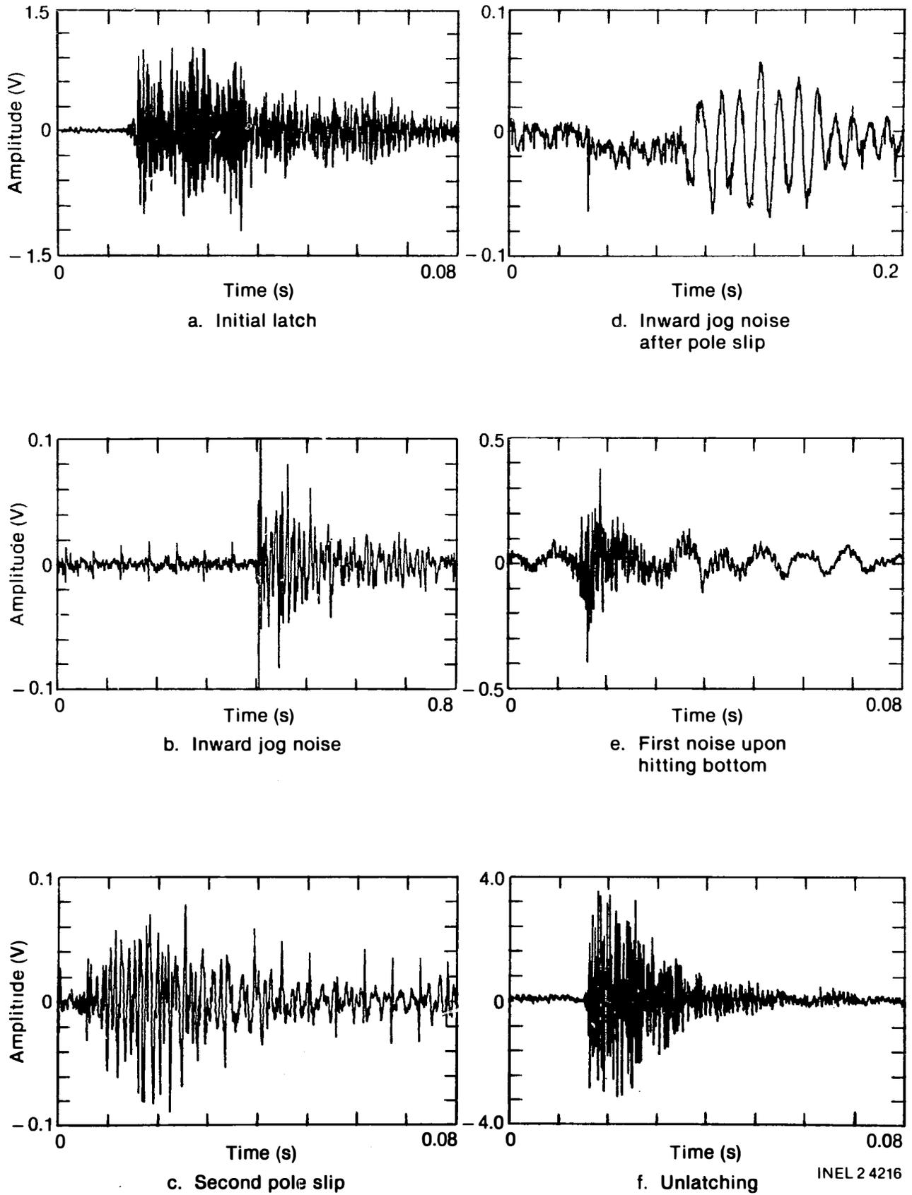
Figure 6. Acoustic signature of selected significant APSR rod movement events, as recorded on APSR 65 during the TMI-2 Insertion Test.
