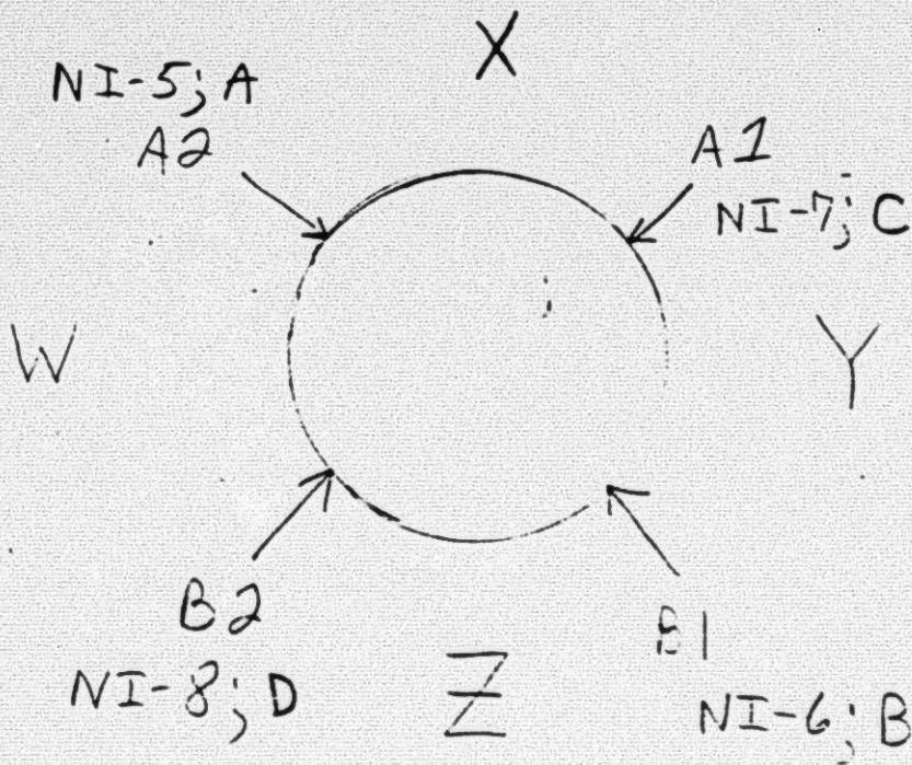
There has been confusion about the arrangements and designations of these detectors and the diagrams should remove this confusion (e.g. the NI-5 UIC detector is also designated as the A detector or by the A2 pump or the WX quadrant).
