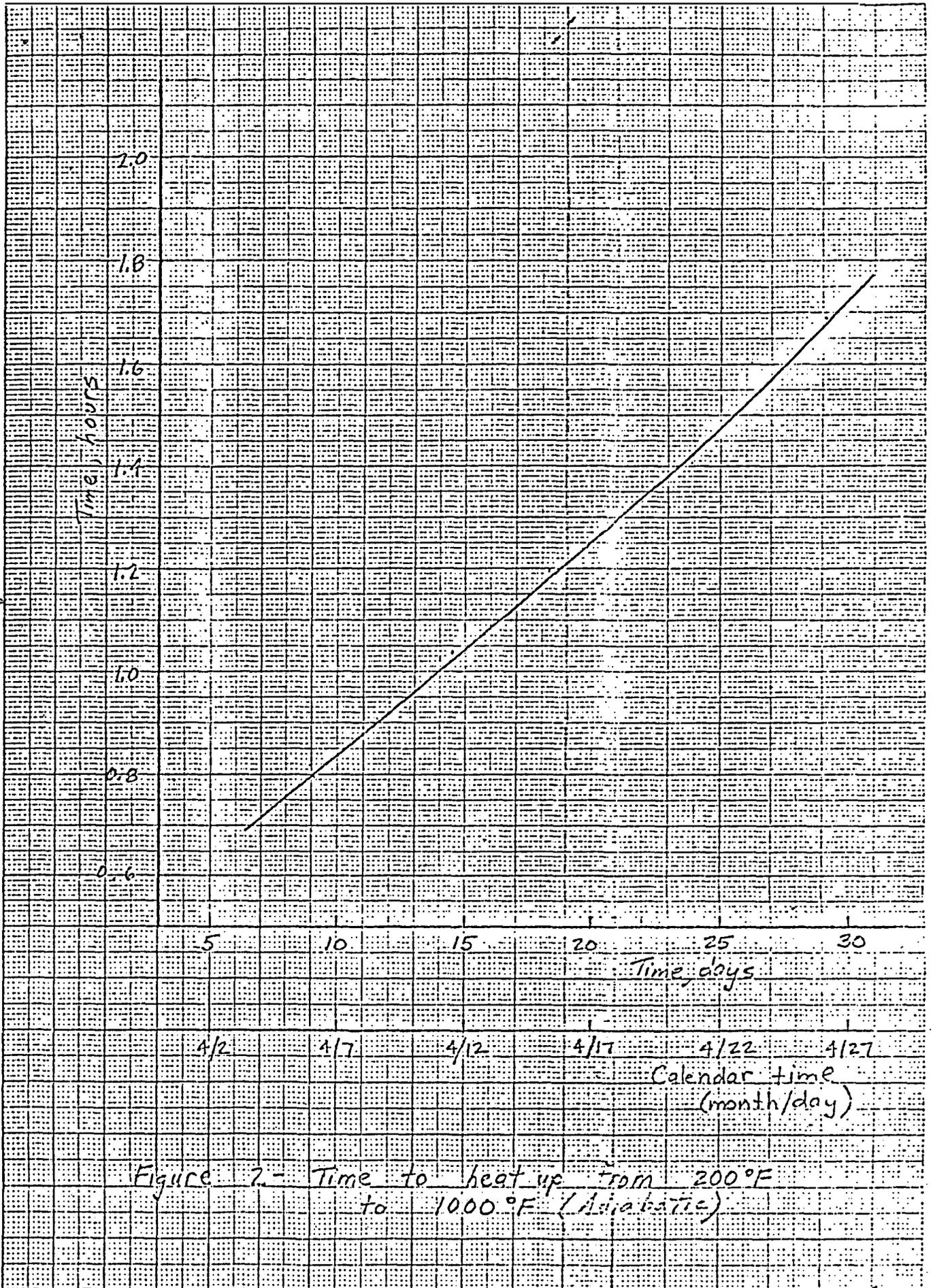
Figure 2.- Time to heat up from 200°F to 1000°F (Adiabatic)
