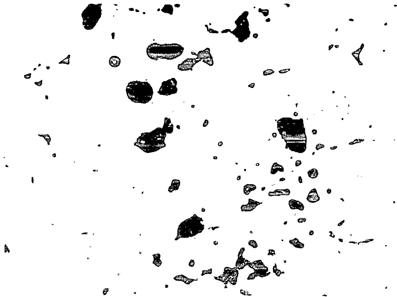
(a) Microphotograph after a heavy etch showing no grain structure.
