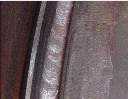
**Fig. 3. Cracks in weld metal**
