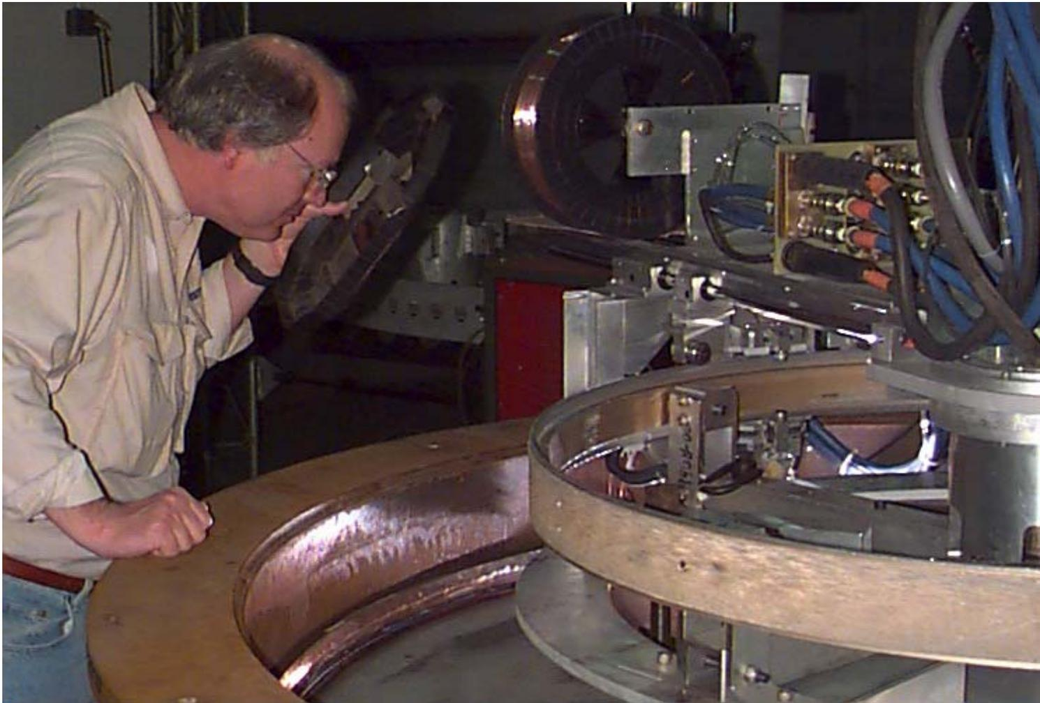
**Fig. 1. Photograph of semiautomatic rotary remote welding system**
