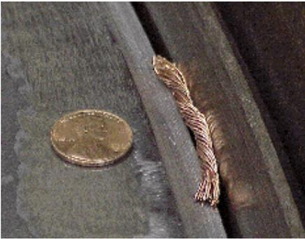
**Fig. 2. Copper wire in joint**
