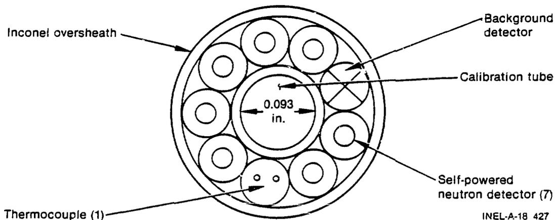
Figure 2. Cross-section of the in-core instrument string.
