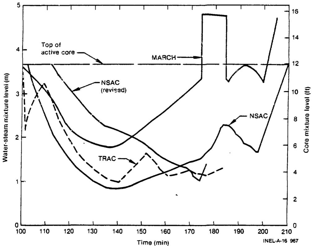
Figure 1. Water-steam and core mixture levels during uncover from 100 to 210 min.
