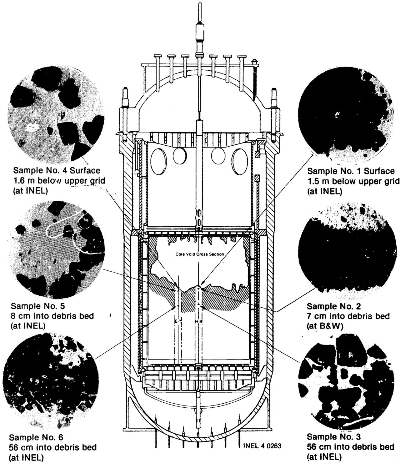
Figure 27. Appearance and location of TMI-2 core debris samples.
