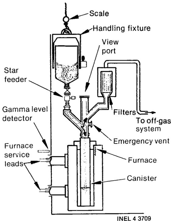
Figure 5. Zeolite vitrification system.
