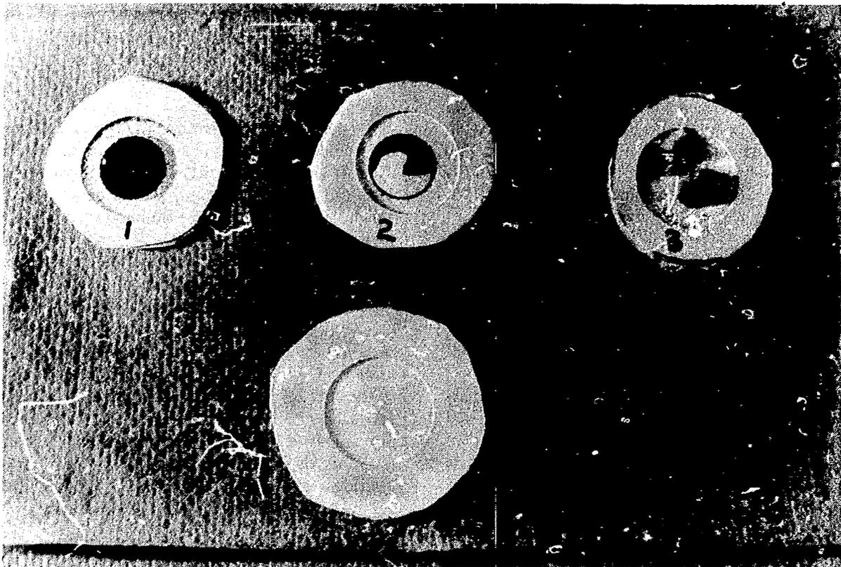
Figure 19. Reactor Building basement filtered solid samples obtained January 11, 1983. The filters are numbered according to sample location, the blank filter is for comparison.
