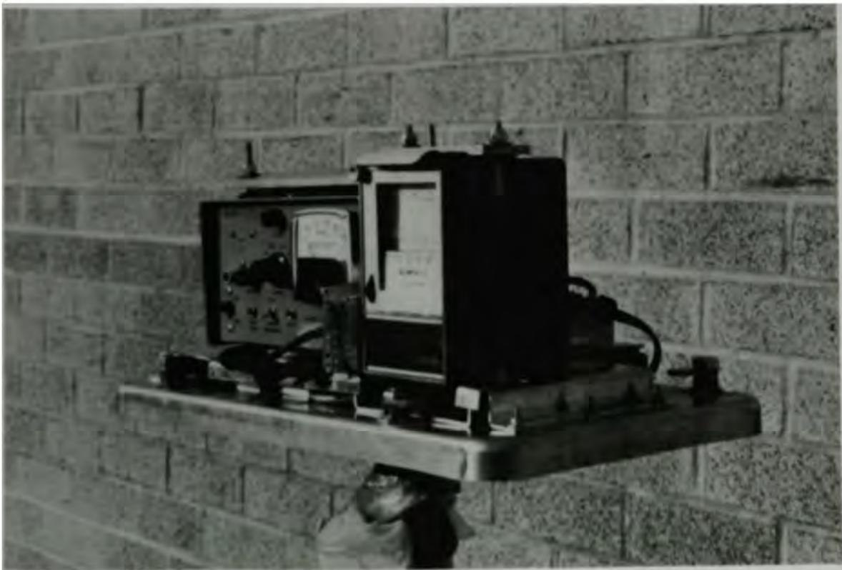
Figure 14. Radiation detector and recorder used in the Citizens Radiation Monitoring Program.
