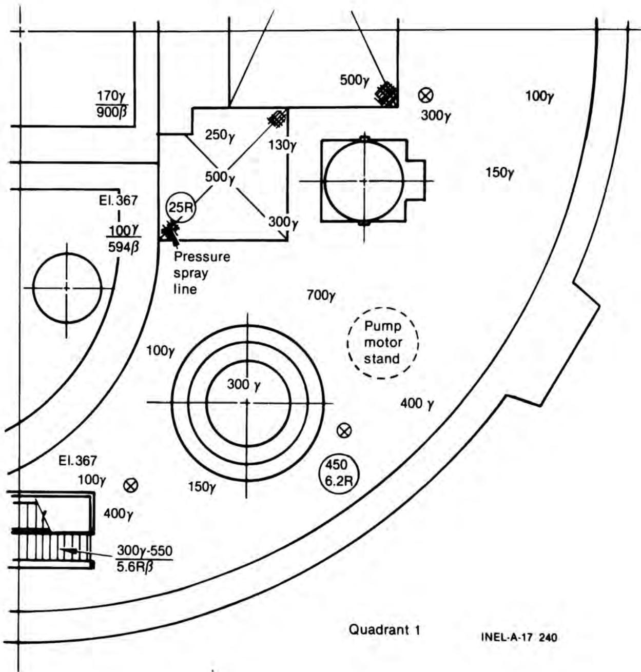
Figure 11. Radiation survey map, 347-ft level.
