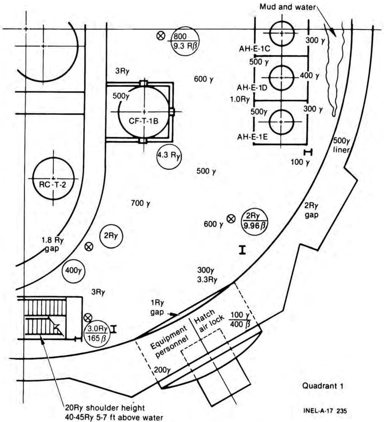
Figure 10. Radiation survey map, 305-ft level.
