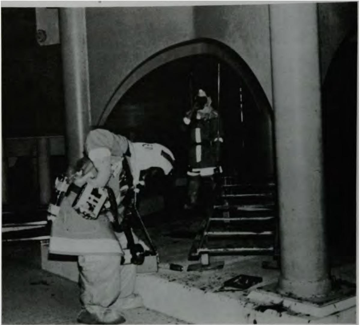
Figure 8. GPU technician taking beta survey at the bottom of the reactor coolant pump stand—July entry.
