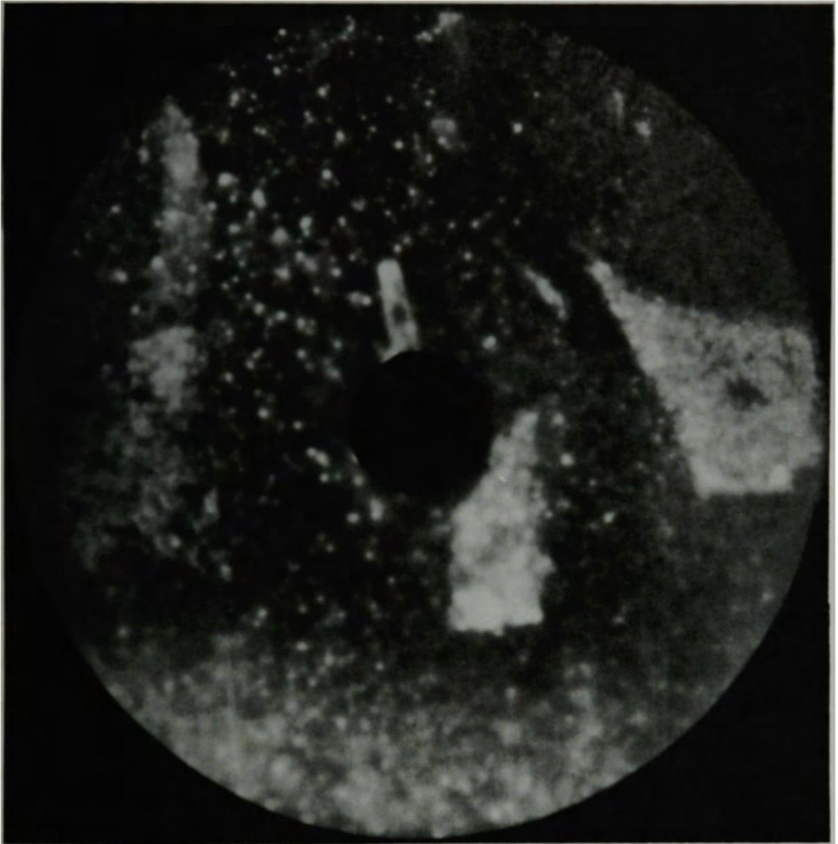
**Figure 5.** Autoradiograph of the contaminated surface of the 9-inch annulus or "cookie".
