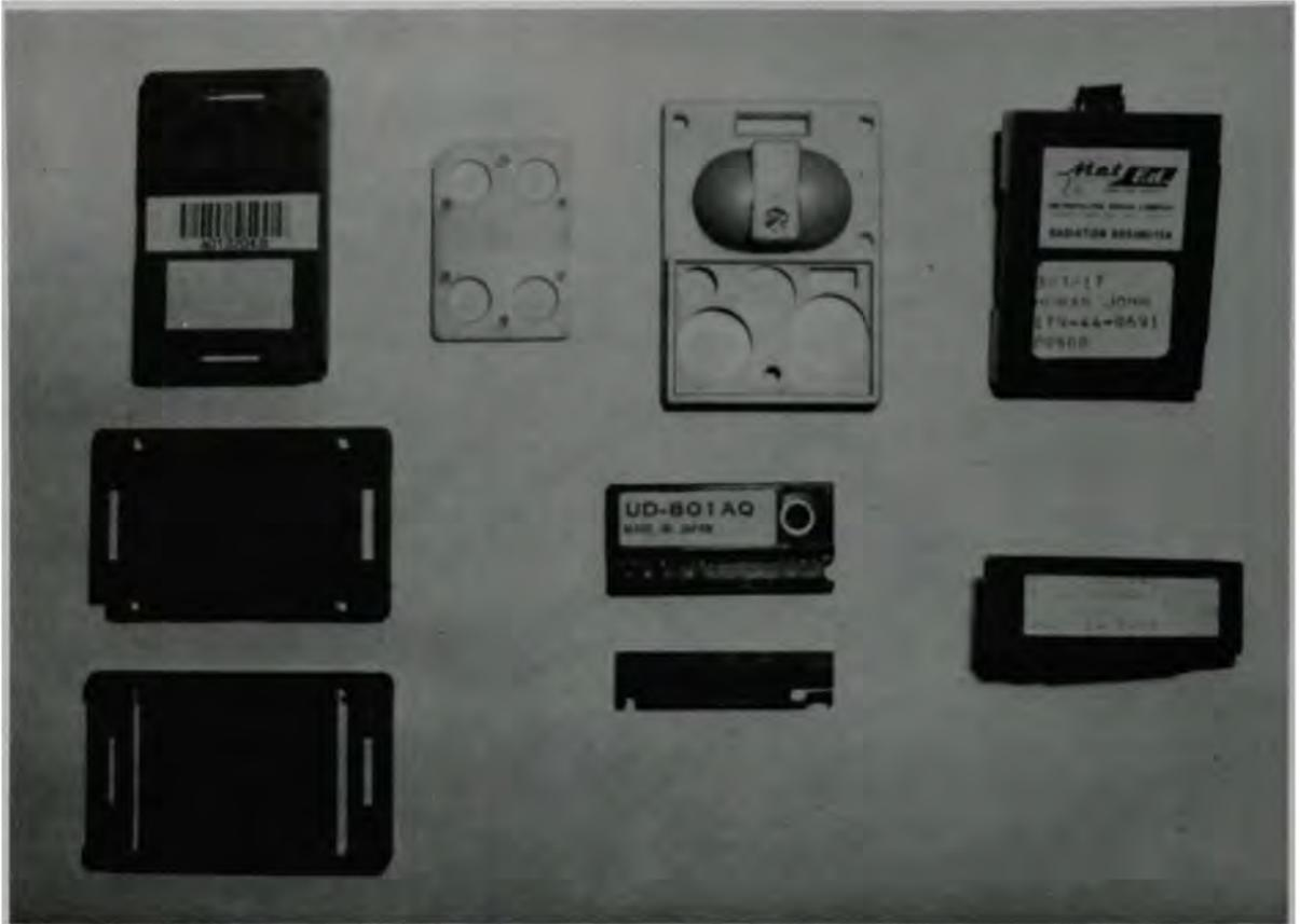
Figure 12. Five different types of dosimeters used during containment entry.
