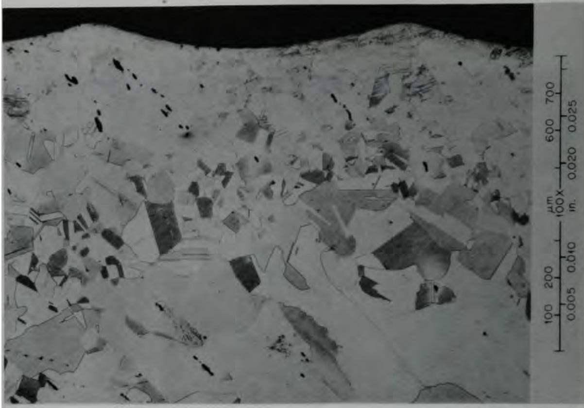
Figure 6. Microstructure of stainless steel "cookie" cross section showing no blast damage.
