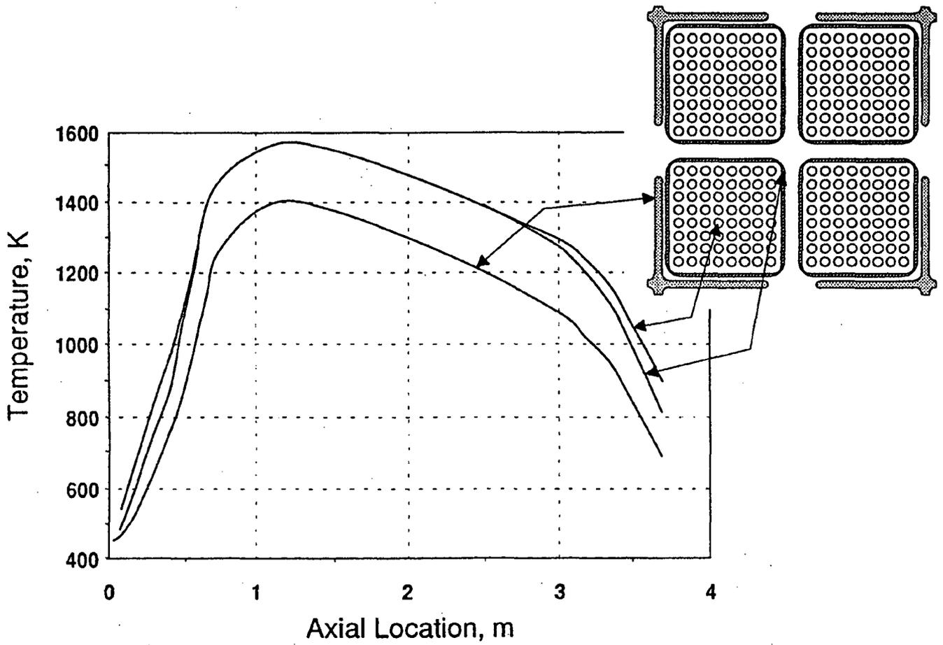
Figure 2.2.2 Axial Temperature Profiles for the Control Blade, Channel Box and Fuel Rods, Indicating Maximum Lateral Temperature Variations
