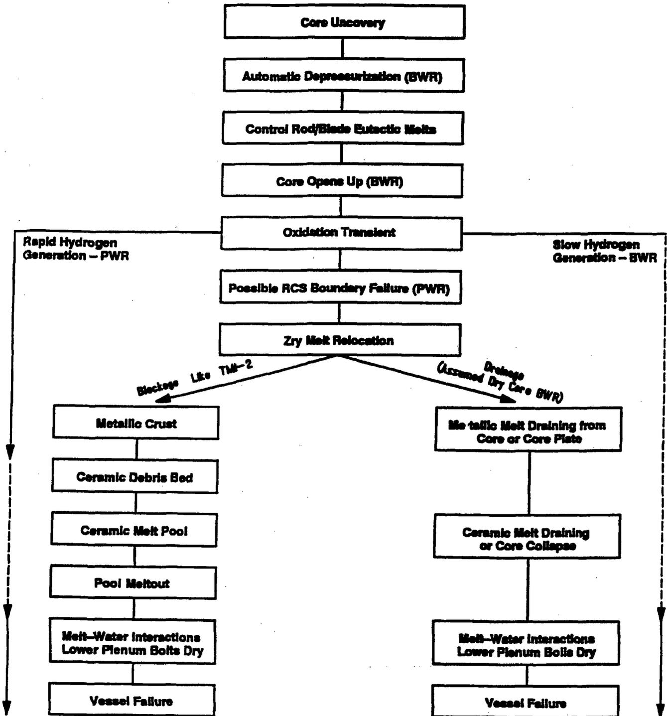
Figure 2.2.1 Core Melt Progression Sequence Showing Blockage or Drainage Paths.
