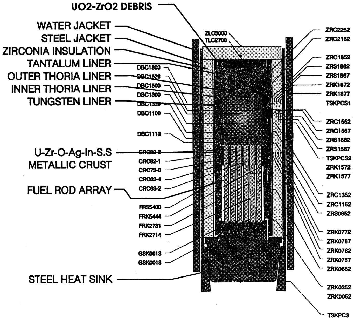
Figure 2.2.6 MP-2 Test Section Showing Major Components and Thermocouple Locations.
