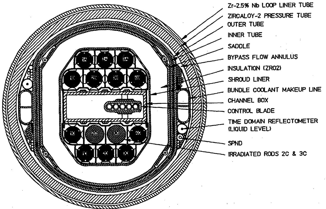
Figure 2.2.5 Test Bundle Cross-Section for the NRU BWR Test
