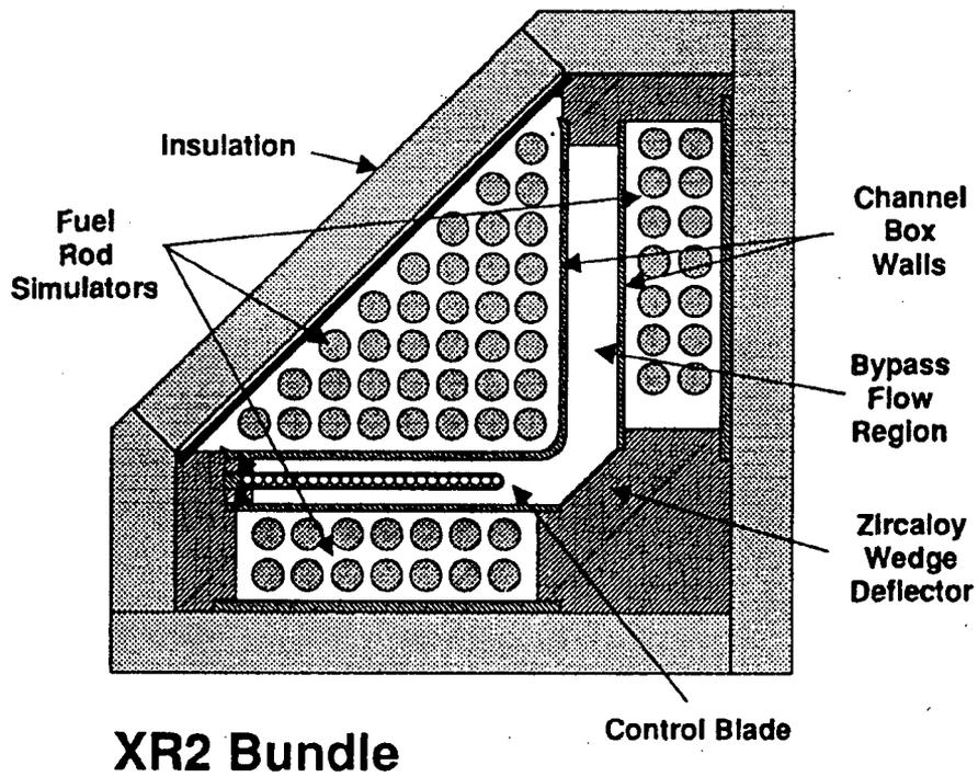
Figure 2.2.3 XR1 and XR2 Test Bundle Cross Sections.
