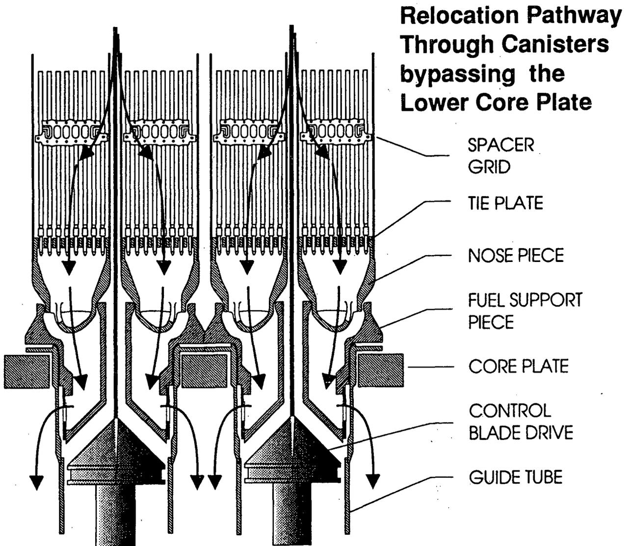
Figure 2.2.4 Melt Drainage Pathways Through the Fuel Canisters Which Bypass the Lower Core Plate.
